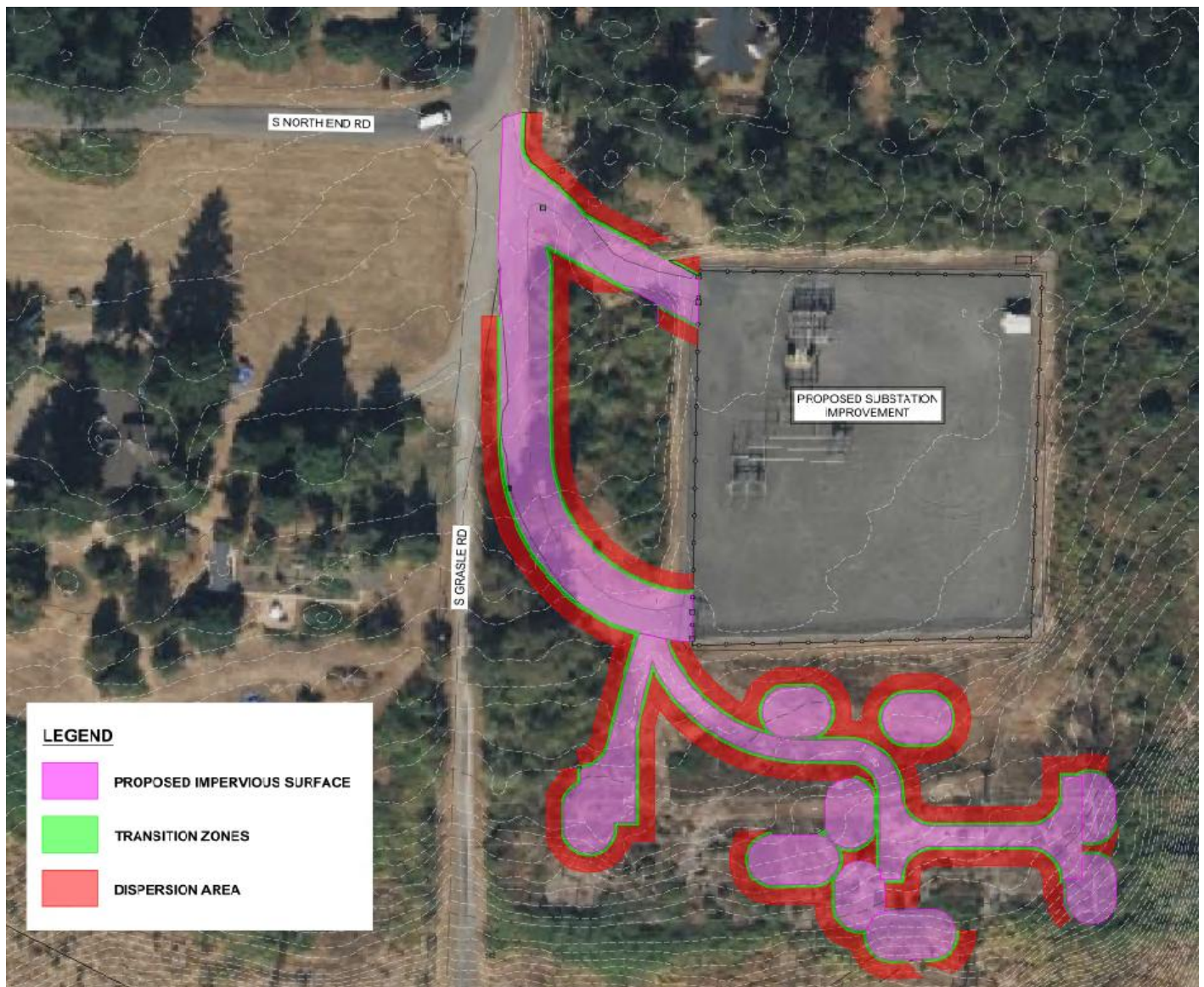
Figure 3. Sheet Flow Stormwater Management Facility.
