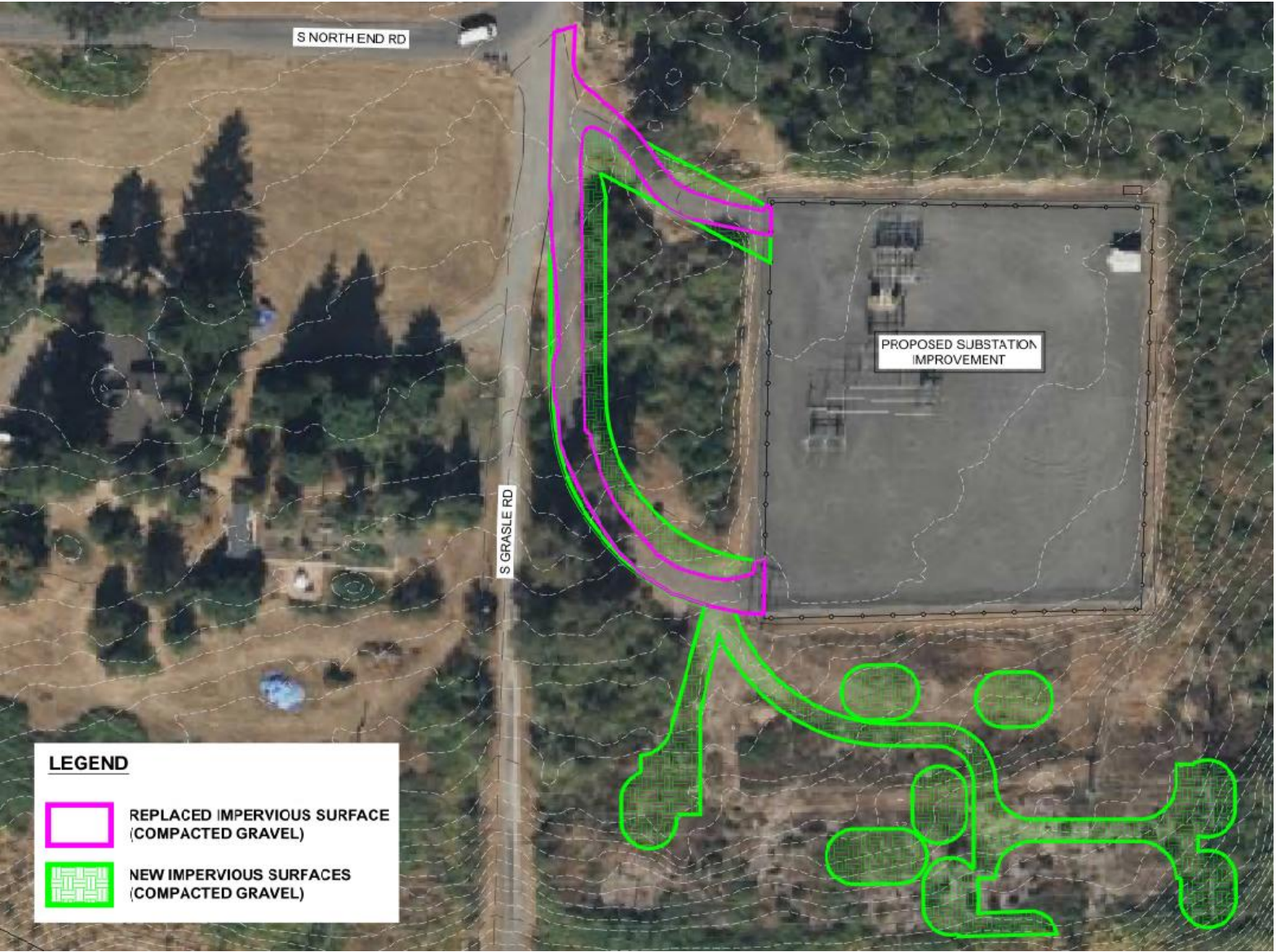
Figure 2. New and Replaced Impervious Area
