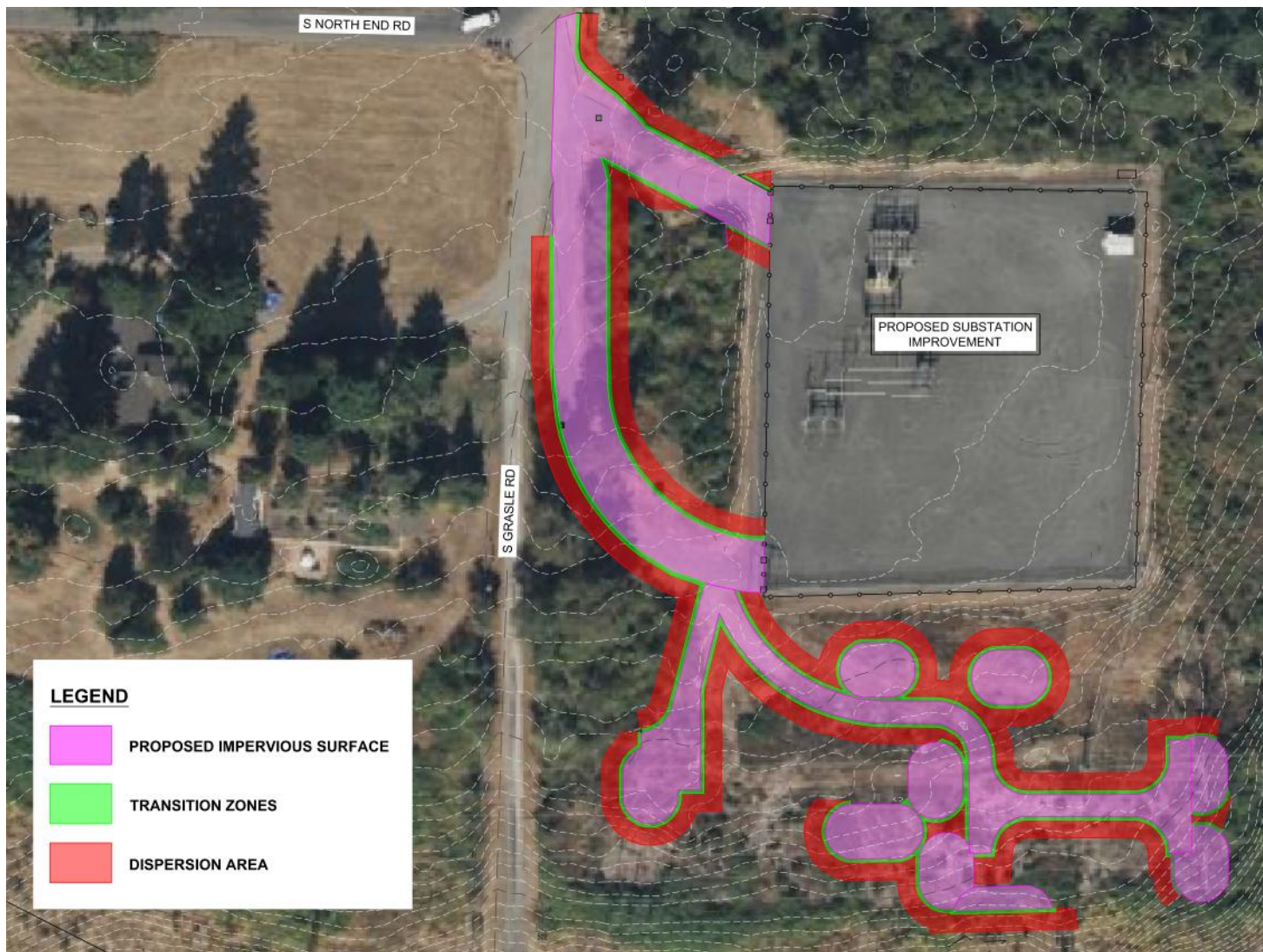
Figure 3. Sheet Flow Stormwater Management Facility.
