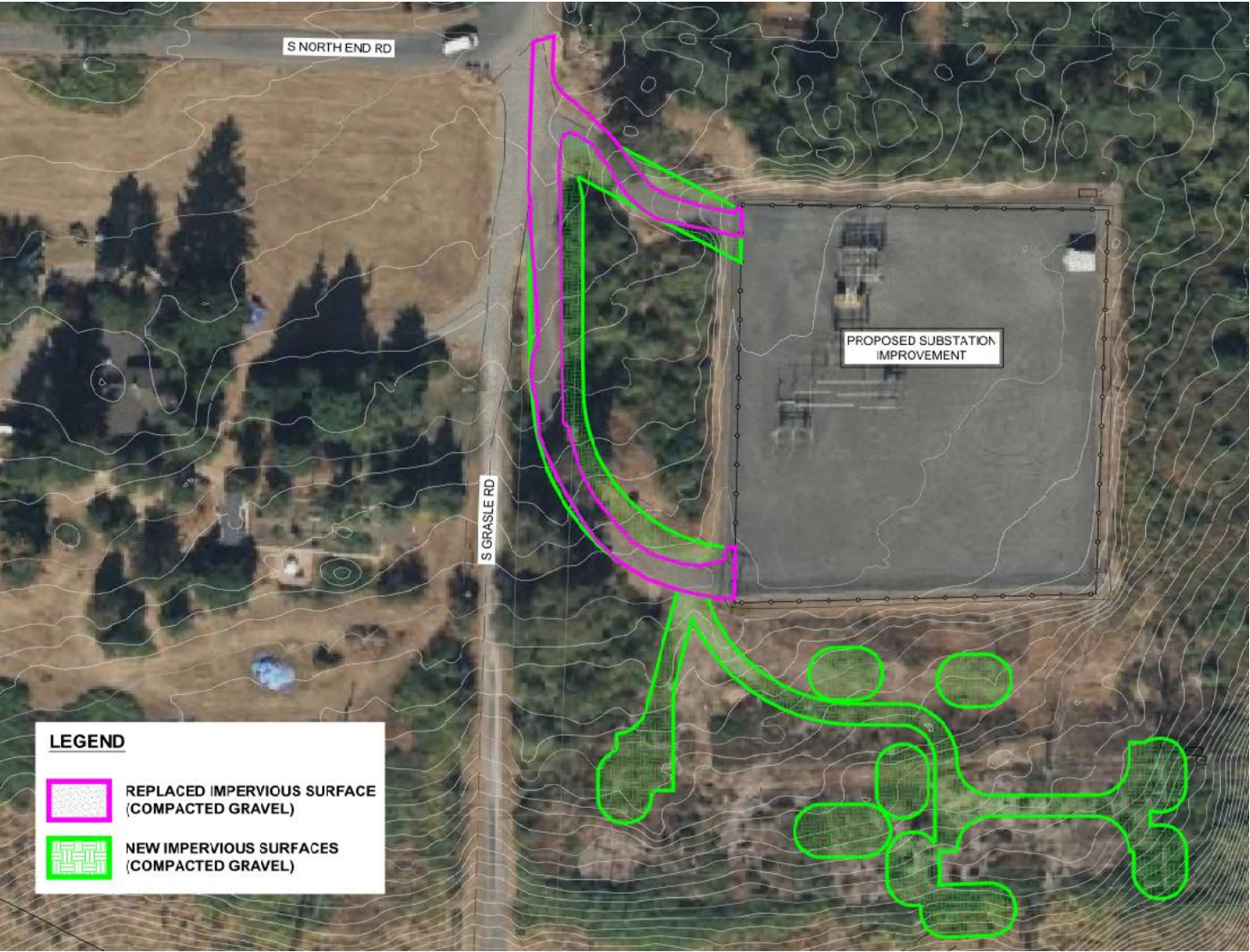
Figure 2. New and Replaced Impervious Area
